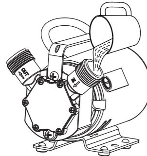
4. Thread a 5/8 in. or larger garden hose (sold separately, max 50 ft. length) to the discharge outlet on the pump.
